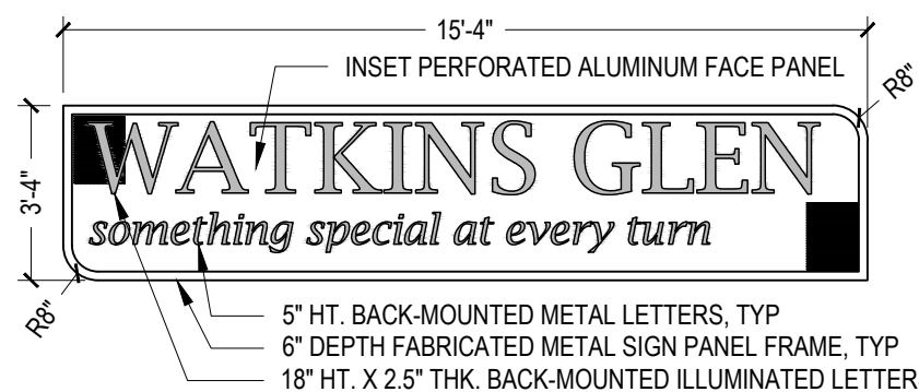
5 NORTH/ SOUTH GATEWAY SIGN PANEL - FRONT ELEVATION - ITEMS 690.01000205/ 690.01000305 Scale: 1/4"=1'-0"
