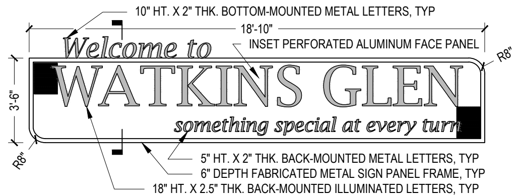
6 EAST GATEWAY SIGN PANEL - FRONT ELEVATION - ITEM 690.01000105 Scale: 1/4"=1'-0"
