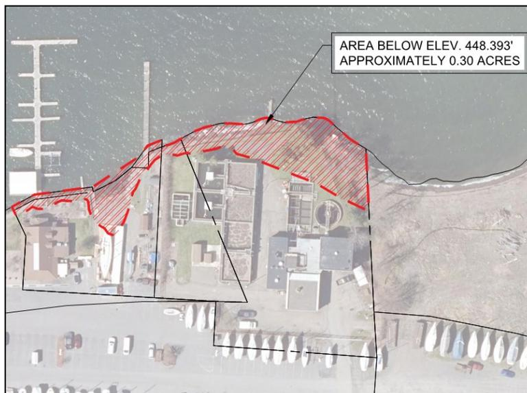
**Figure 3.2.1:** Excerpt of Floodplain Mapping Analysis
