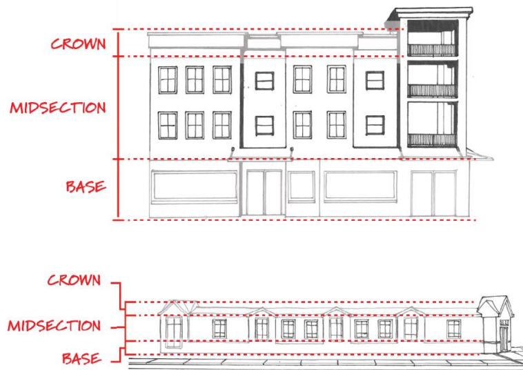
FIGURE 32.2 TRIPARTITE (3-PART) FAÇADE DESIGN
