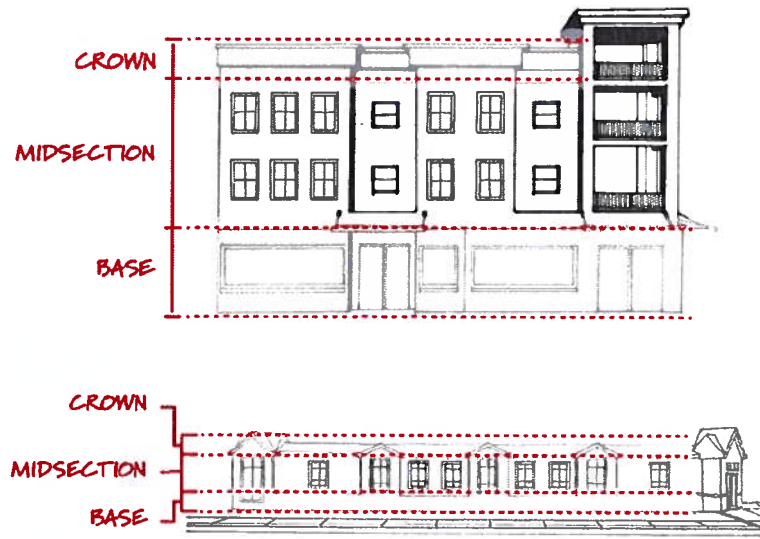
FIGURE 32.2 TRIPARTITE (3-PART) FAÇADE DESIGN
